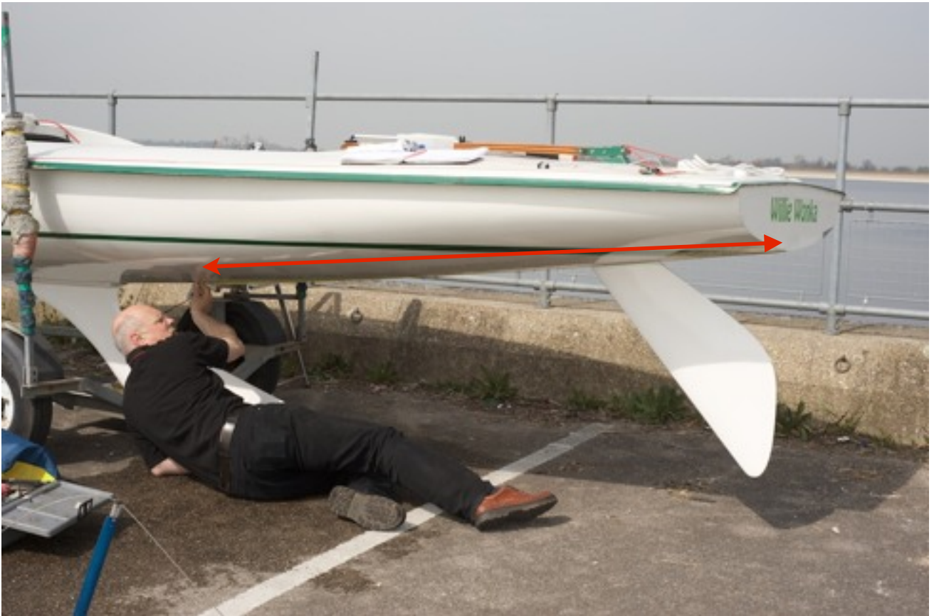
Measuring from transom to bailer outside the hull
